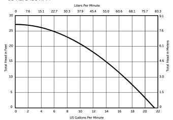
For proper performance, tank inflow cannot exceed pump discharge capacity at the installed head level.
