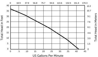
Note: Maximum shut-off head is 36'. Usable maximum head - assuming 150' of lateral discharge through 1"—pipe is 25'. Consult factory for proper sizing and calculation of friction loss.
