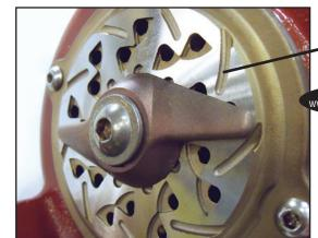
**Exclusion cleanout** slots and back relief clears debris from under cutter
